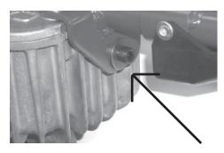
DO NOT re-use the lock washers when fastening the 4 top clamp bolts, instead, use the hardened flat washers included in the fastener kit. Be sure to use the 1-1/4" long bolts on the left side and the 1-1/2" bolts on the right side and torque properly to 24 ft-lbs.
