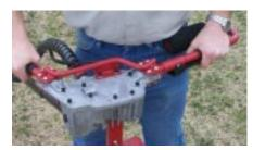
It is essential that the five bolts which mount each handle to the transmission be kept tight at all times. Loose bolts, especially item A below will allow the aluminum cover plate to flex during operation and will lead to breakage.
