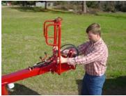
Fold handle into operating position. Machine can also be operated with handle in the rearward position for drilling next to a wall.
