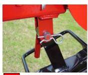
11 Attach tow bar by slipping under reservoir and lifting over hooks. Lift up, attach pin & secure with clip.
