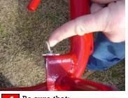
4 Be sure that: The stop switch on the handle is ON. The stop switch on the engine is ON. The fuel valve is ON.
