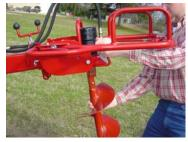
Release latch & attach auger. (Machine may be moved w/ auger attached & locked.) Move into position & adjust side-to-side position if necessary.
