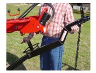
Unhook tow bar from 2" ball (vehicle). Remove tow bar from machine.
