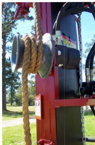
3 Wrap rope approximately 2 turns around cathead as shown.
