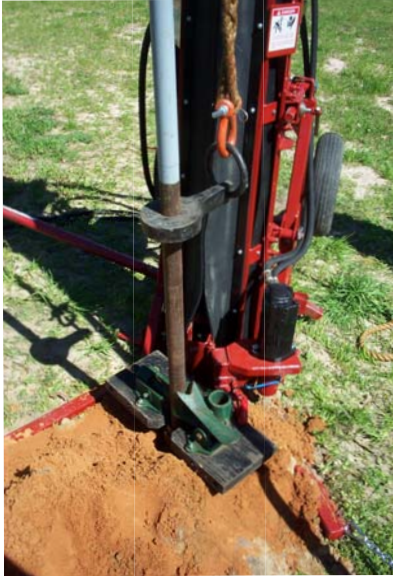
6 Several optional tools (such as lift ring and clamp as shown above) are available to aid in sampling especially at greater depths.
