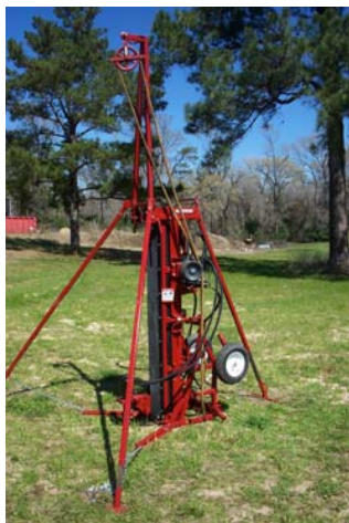
10 Drill to sampling depth. Refer to Big Beaver Operator's Manual and/or Hollow Stem auger Instructions for proper drilling procedure.
