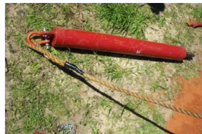
2 Connect rope to safety hammer (140 lb. max) using clevis and pin.
