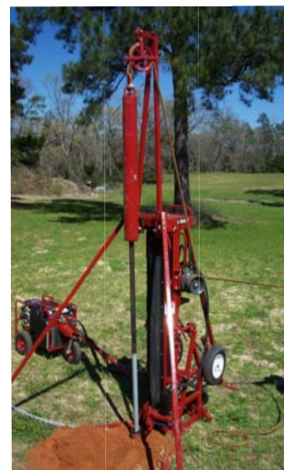
5 Begin sampling as required by raising and dropping the 140 lb. hammer. The Standard Penetration Test (SPT) may be performed as described in the standard ASTM D 1586.
