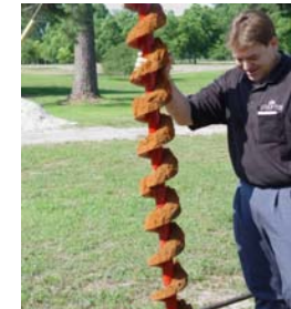
12 Remove handle, then remove auger and extension from hole.
