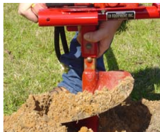
9 For greater depths, un-snap auger from auger adaptor.
