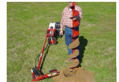
12 Remove handle, then remove auger and extension from hole.
