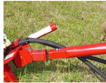
2 Snap male end of torque tube into connector at handle.
