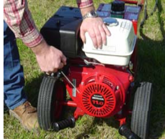
5 Then pull starter rope. Note: engine should always run at full speed.
