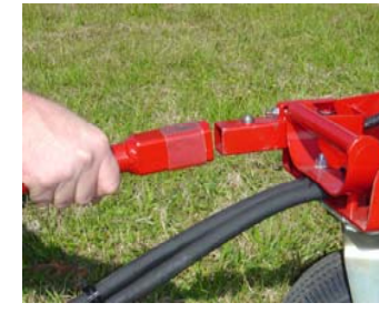
3 Snap female end of torque tube into connector on power source.
