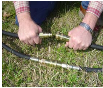
1 Connect handle to power source using quick disconnect fittings.
