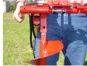
6 Attach auger to auger adaptor.
