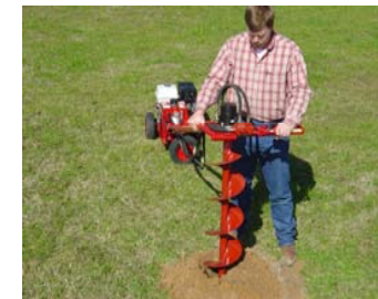
11 Continue digging with auger and extension.
