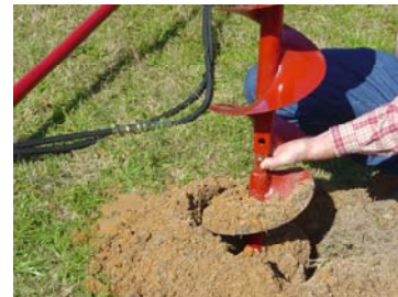
10 Snap extension onto auger.
