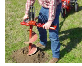
7 For safety, always keep leg pad against leg while digging.
