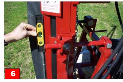
6 Level the drill mast by referring to the Big Beaver operator's manual.
