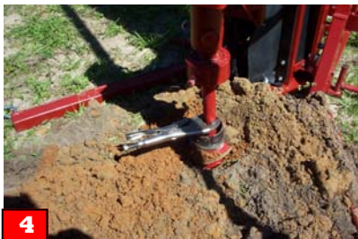
4 Loosen drive cap locking bolts (2). Raise drive cap while remaining connected to center rod. While using locking pliers as a stop to hold the center rod, lower drive cap and center rod until adaptor pin moves freely.
