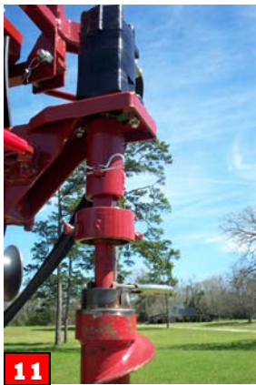
11 Pivot and lock drill head into place. Connect drill head to drive cap using adaptor pin.
