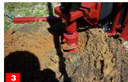
3 Drill to bottom of stroke or desired sampling depth. Without rotating, raise and/or lower drill string until cutter head is resting on the bottom of the hole (the adaptor pin can be moved freely).
