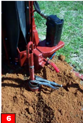
6 Pivot drill head to side. Attach center rod puller to top of center rod with drive pin.
