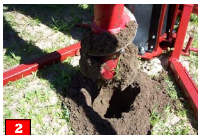
2 If drilling through sod or heavy ground cover, raise auger to clear debris from cutter head before continuing.
