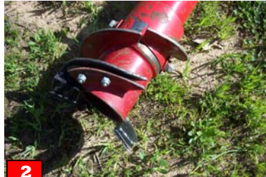
2 Attach cutter head by aligning the keys with the slots and tightening the (2) locking bolts.
