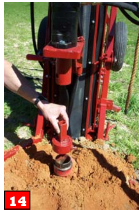
14 When drilling has been completed, remove all center rod from hole. Attach drive cap to hollow stem.
