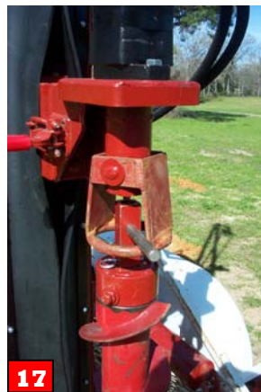
17 If necessary, the auger string may be rotated when retrieving.
