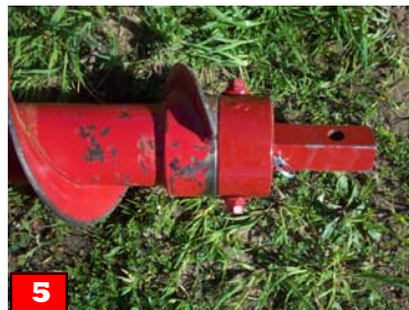
5 Attach drive cap by aligning the keys with the slots and tightening the (2) locking bolts.
