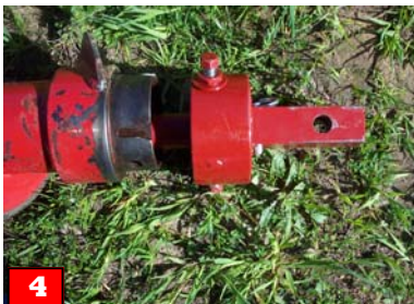
4 Attach drive cap to center rod with pin.
