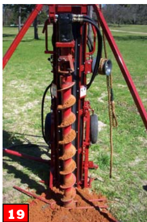
19 Lower auger string until its weight is supported by the auger fork/stop.
