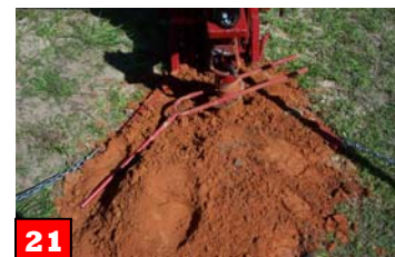
21 Reattach drive cap to auger string. Use retrieval pin to connect drive cap. Raise auger string to remove auger fork/stop.
