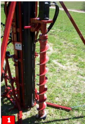
1 Attach lead auger assembly to drive adaptor using the adaptor pin. Lower lead auger assembly, without rotating, until the point contacts the ground. Be sure auger is parallel with the drill mast. Begin drilling.
