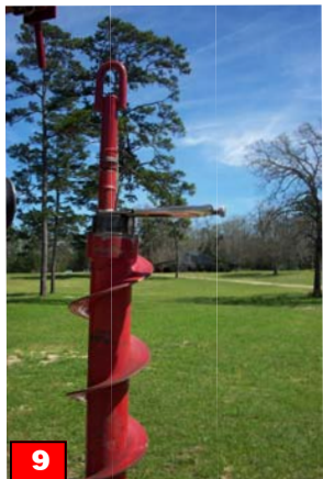
9 Add hollow stem section by sliding over center rod and attaching to hollow stem string. Use locking pliers as stop to hold center rod above hollow stem.
