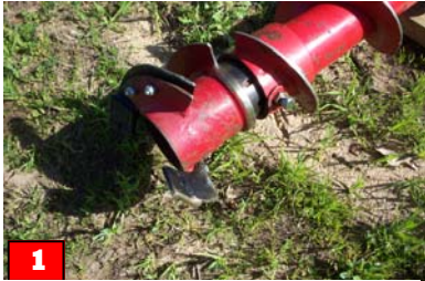
1 Loosen the (2) locking bolts to allow cutter head to be assembled to the bottom of hollow stem auger.
