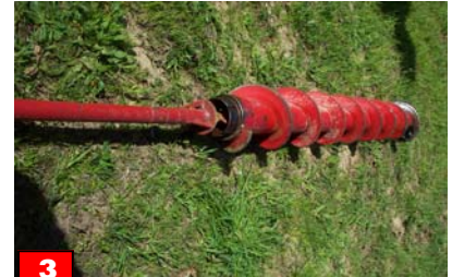
3 Insert center rod with point and plug attached..
