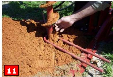
11 Disconnect extension bottom by removing pin.
