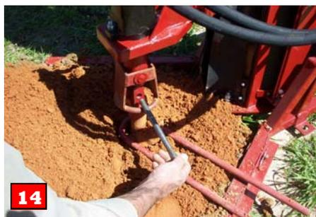
14 Lower retrieval ring over auger (extension) top and connect with pin. Remove auger fork (stop) after auger string is secured by retrieval ring.
