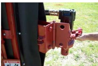
**NOTE:** It may be beneficial to pivot drill head to the side when adding or removing extensions.
