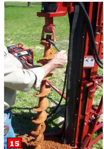
15 Continue procedure until lead auger is removed.
