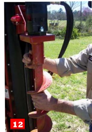
12 Raise drill head. Disconnect extension top by removing pin.
