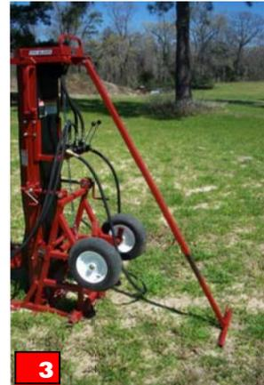
Lift back stay base. Pivot and extend back stay into position.
